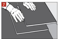
Place the plank to be repeated exactly on the last installed row of planks. Then mark the longitudinal section using another plank. This type of marking leaves sufficient distance to the wall in order to angle the last row by means of pull bar.
