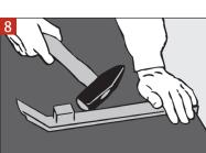
8 The last row of planks is rounded on the side with the pull bar and on the front side with the ZIRO tapping block.
