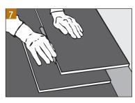
7 Fitting the last row of planks: Place the plank to be repeated exactly on the last installed row of planks. Then mark the longitudinal section using another plank. This type of marking leaves sufficient distance to the wall in order to angle the last row by means of pull bar.
