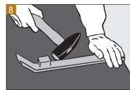
The last row of planks is rounded on the side with the pull bar and on the front side with the ZIRO tapping block.
