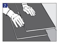
7 Fitting the last row of planks: Place the plank to be repeated exactly on the last installed row of planks. Then mark the longitudinal section using another plank. This type of marking leaves sufficient distance to the wall in order to angle the last row by means of pull bar.
