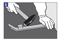
8 The last row of planks is rounded on the side with the pull bar and on the front side with the ZIRO tapping block.
