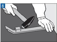
B The last row of planks is rounded on the side with the pull bar and on the front side with the ZIRO tapping block.
